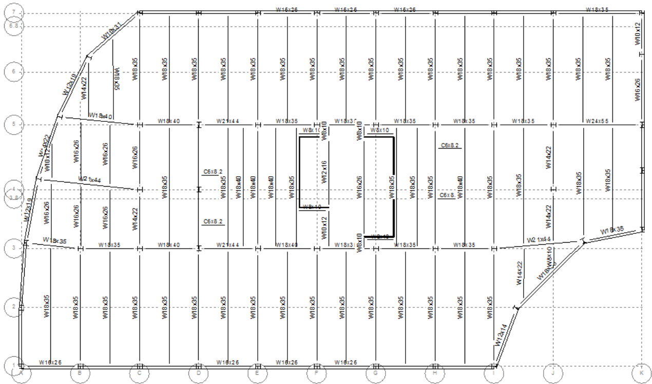
Figure 16: Typical Redesigned Office Framing Plan
